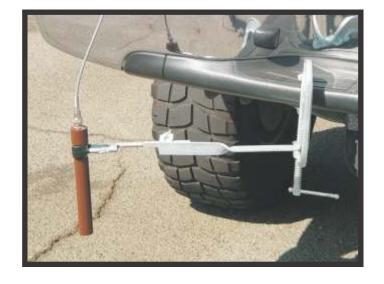
Clamp holds probe in 90° and 45° angles for pipeline locating, center and depth determination
